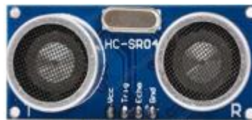
Fig. 5: HC-SR04 - ultrasonic sensor
